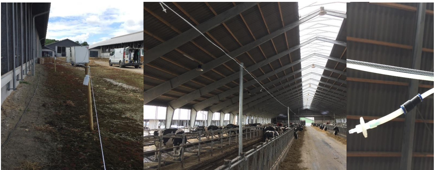
Figur 5 sample lines outside and inside the barn. To the right a sampling point equipped with a critical orifice, and a dust filter
